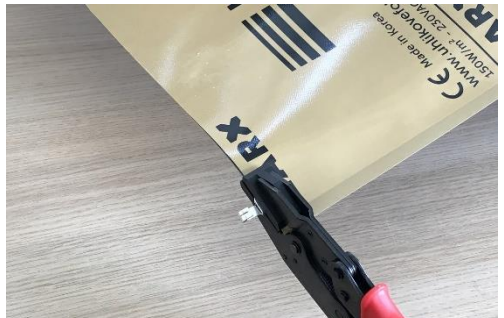
Connector pressing by clamp pliers
